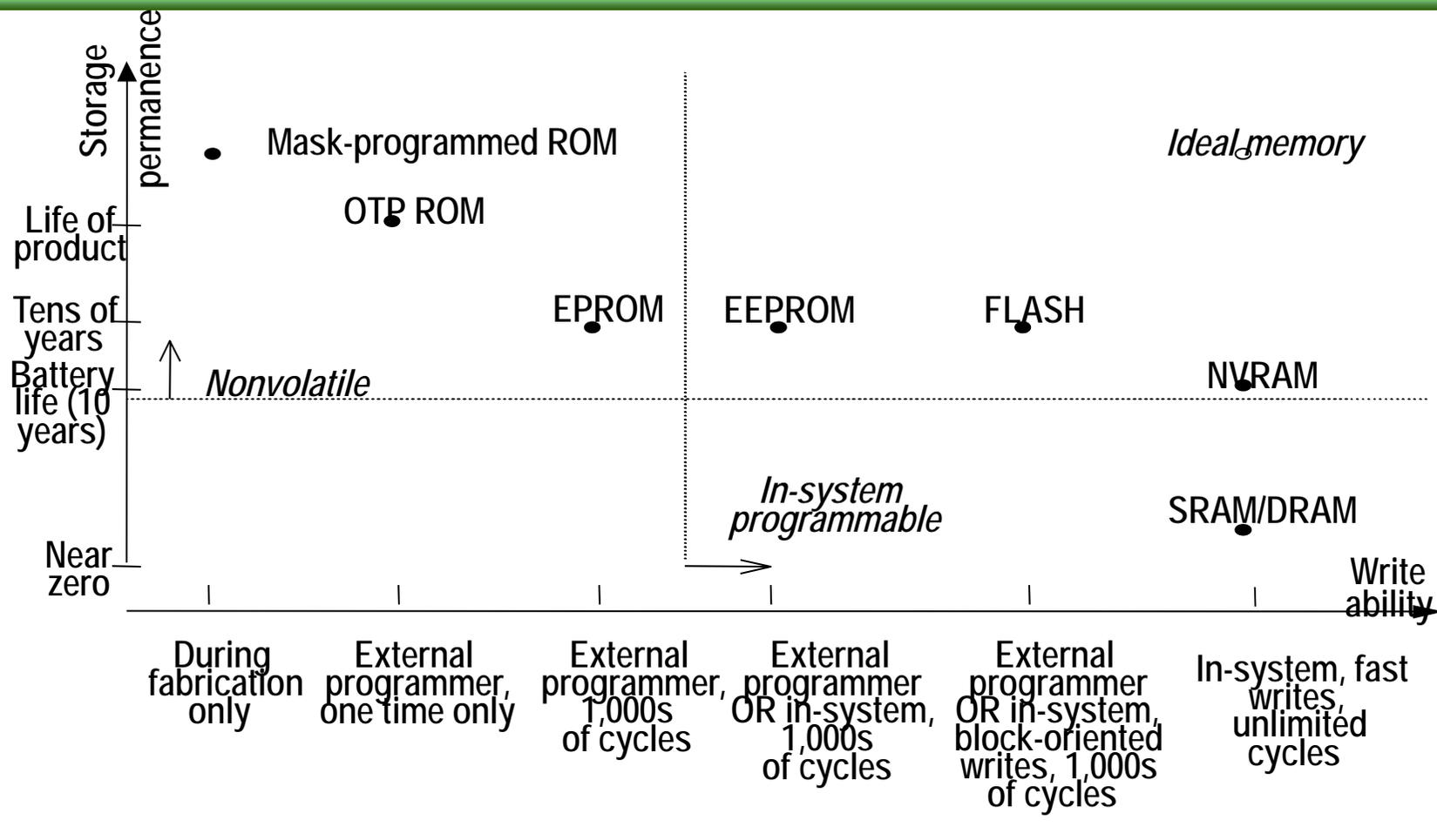
Write ability and storage permanence of memories, showing relative degrees along each axis (not to scale).
